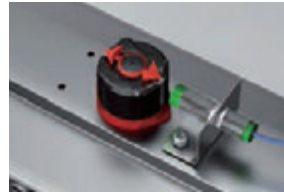
Inductive switch indicating open or closed position
